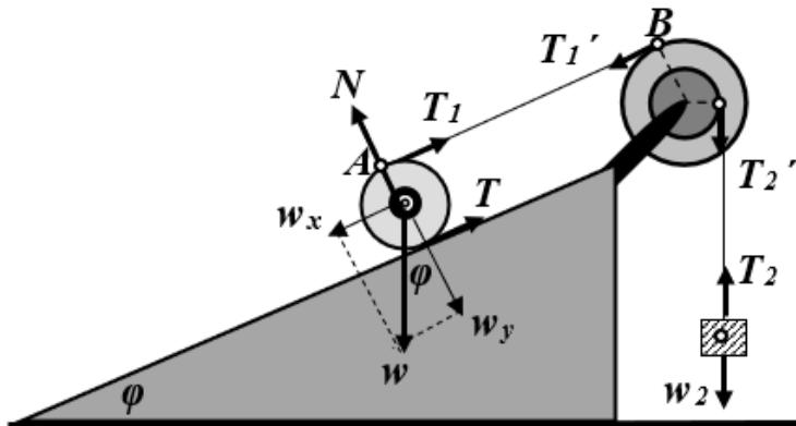
$$\Sigma \tau_{ερεό} \Pi: \Sigma \tau = 0 \Rightarrow T_1' \cdot 2R - T_2' \cdot R = 0 \Rightarrow T_2' = 2 \cdot T_1' \xrightarrow{T_1' = T_1 = 15N} T_2' = 30N$$
