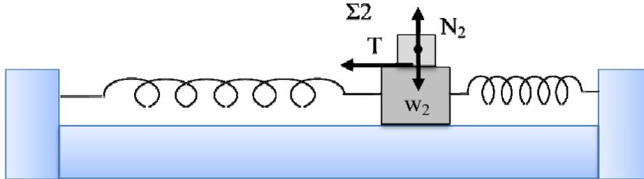
$$\left. \begin{aligned} \Sigma F_x &= -D_2 \cdot x \\ \Sigma F_x &= -T_\sigma \end{aligned} \right\} \Rightarrow T_\sigma = D_2 \cdot x = m_2 \cdot \omega'^2 \cdot x$$
