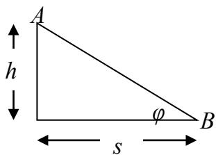
$$\varepsilon\phi\phi = \frac{h}{s} \xrightarrow{(3) \Rightarrow h = \frac{1}{2}gt_{o\lambda}^2 \text{ & (1)} \Rightarrow s = v_2 t_{o\lambda}} \varepsilon\phi 30^\circ = \frac{\frac{1}{2}gt_{o\lambda}^2}{v_2 t_{o\lambda}} \Rightarrow t_{o\lambda} = 0,2\sqrt{3} \text{ s ,}$$
