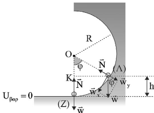
$$E_{M,Z} = E_{M,\Lambda} \quad \text{ή} \quad K_Z + U_Z = K_\Lambda + U_\Lambda \quad \text{ή} \quad \frac{1}{2} m_3 v_3^2 + 0 = 0 + m_3 g h \quad \text{ή} \quad h = \frac{v_3^2}{2g} \quad \text{ή} \quad h = 0,2 \text{ m}$$
