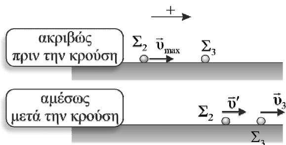
$$\vec{p}_{o\lambda(\pi\rho\nu)} = \vec{p}_{o\lambda(\mu\varepsilon\alpha)} \quad \& \quad m_2 \cdot v_{\max} + 0 = m_2 \cdot v' + m_3 \cdot v_3 \xrightarrow{(1)} v' = 0$$
