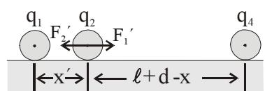
$\therefore \frac{|q_1|}{x'^2} = \frac{|q_2|}{(d + \ell - x')^2} \quad \therefore \frac{1.10^{-6} \mu\text{C}}{x'^2} = \frac{4.10^{-6} \mu\text{C}}{(4-x')^2}$
