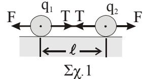
$$T = 9 \cdot 10^9 \text{ N.m}^2/\text{C}^2 \frac{1 \cdot 10^{-6} \mu\text{C} \cdot 4 \cdot 10^{-6} \mu\text{C}}{(2m)^2} \quad \text{ή } T = 9 \cdot 10^{-3} \text{ N}$$
